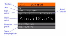
The new SMART EBULLIOMETER has a modern and intuitive graphic interface and provides, in addition to boiling temperature, directly also the value of the alcohol content!!
